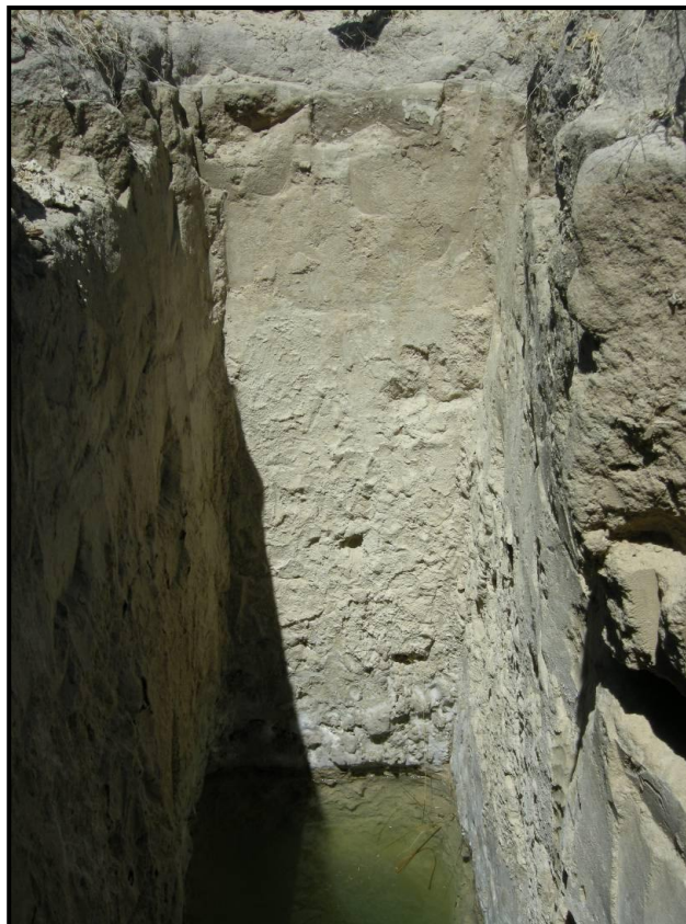
Figure 32: Excavation showing the depth of the water table at about 2m below the surface.
