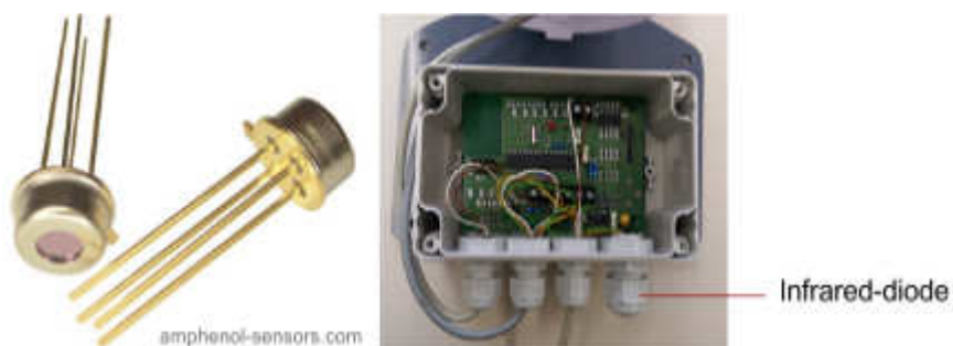
Figure 17: Infrared-sensor as a single compound (l) and installed (r).
