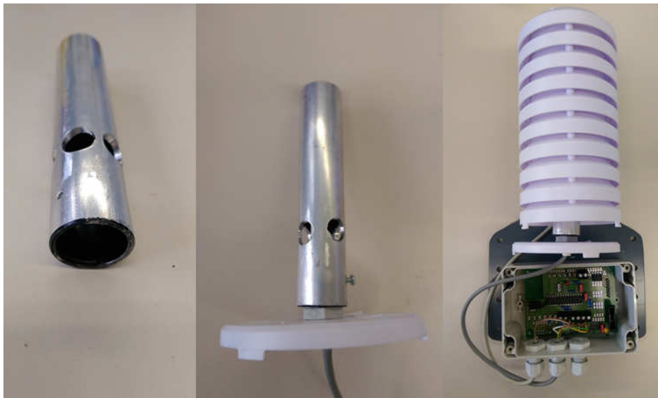
Figure 15: Aluminum-tube attached to the radiation shield to get more accurate data.
