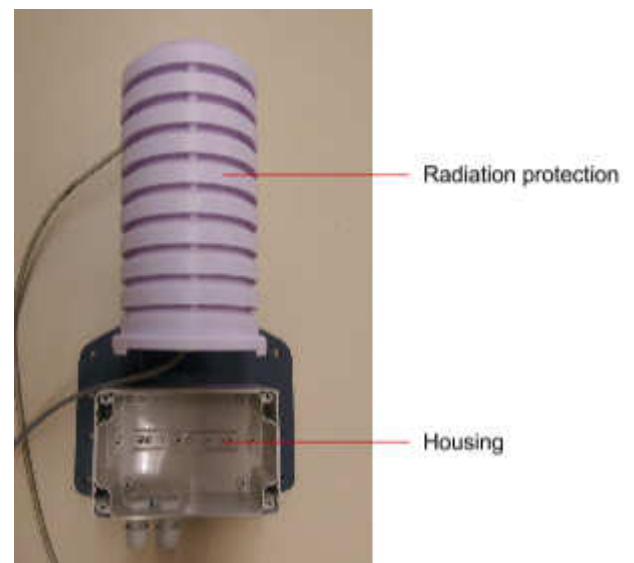
Figure 14: Radiation protection fixed on a PVC-base.
